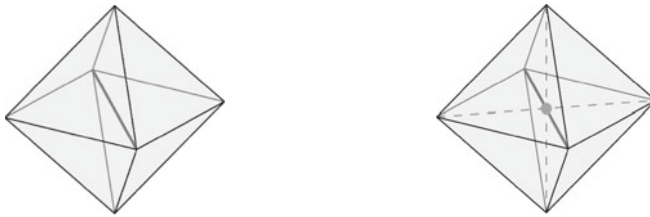
(a) A compatible patch \omega_e with common edge e (b) Patch \omega_p after a compatible bisection b_p
